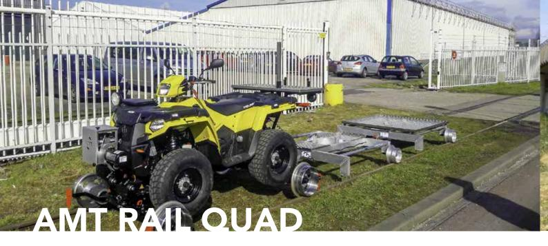
MT railroad ATV's are designed to make working on and around the track more efficient and easier.
