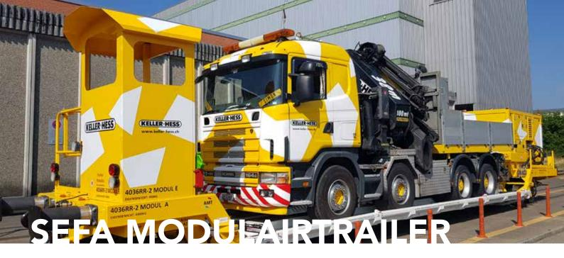
Together with our Swiss Partner Ramorailso AG, AMT developed a special railtrailer which is modulair for transporting special vehicles or loads on the rail.
