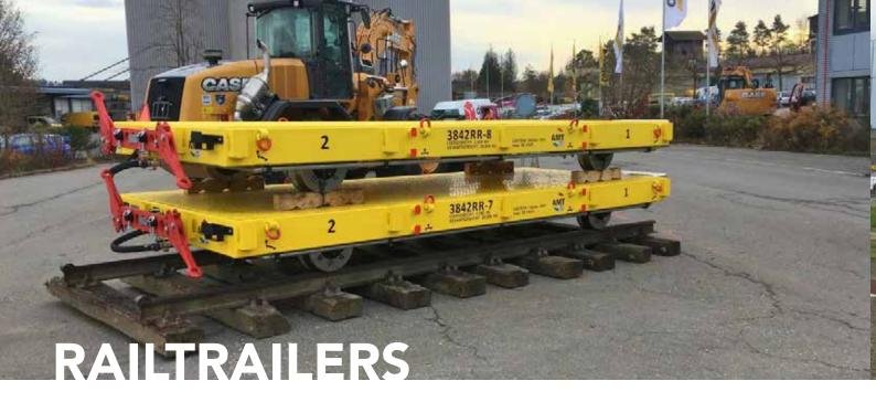
AMT railtrailers are designed to allow you to work as efficiently as possible. The trailers are built according to customer specifications. The compact, low construction and low unladen weight allows for optimal use of the capacity. The robust frame, heavy-duty bearings, and reliable brakes ensure minimum maintenance requirements.
