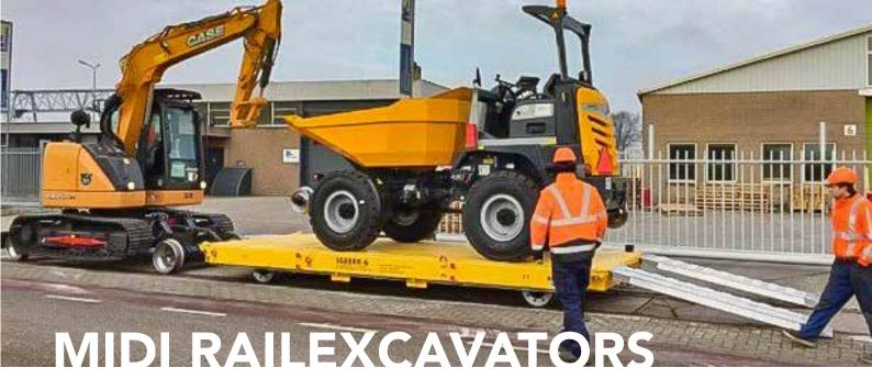
CASE's versatile CX75 & CX145 crawler excavators are equipped with a permanently mounted, hydraulically driven track system for metre, standard, or tram gauge.
